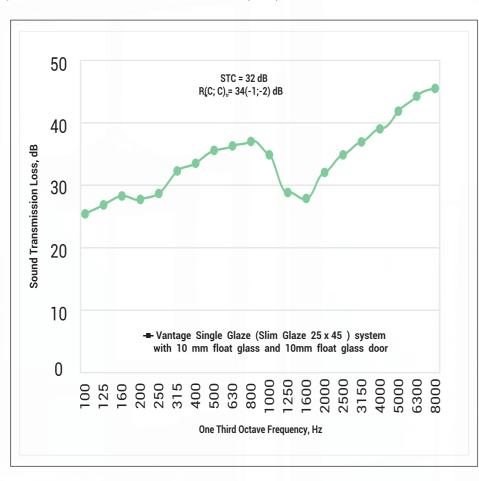
The sound transmission class (STC) is calculated as per ASTM E-413 and weighted sound reduction index with spectrum adaptation terms R<sub>w</sub>(C 100-5000) is calculated as per ISO 717-1
